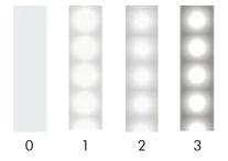
The dot level shows the intensity of hotspots in the combinations of Hilite LED tape light and channels with a frosted diffuser.
