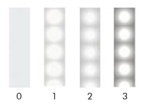
The dot level shows the intensity of hotspots in the combinations of Hilite LED tape light and channels with a frosted diffuser.
